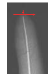
X ray film shows under-filling
